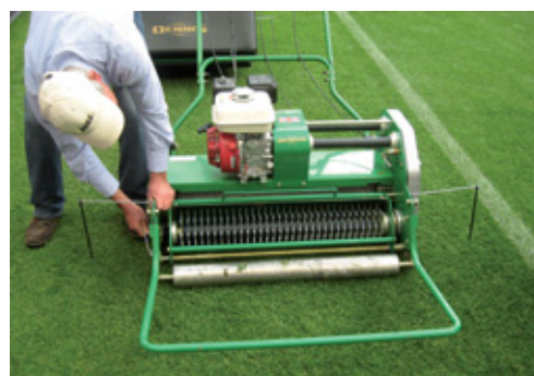
Cylinder mower with verticutting cassette
